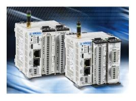
For systems with even higher I/O needs, the 2-slot CPU can also be expanded with up to 8 additional stackable I/O modules for up to 156 discrete I/O or 60 analog I/O points total. Numerous stackable modules are available, offering discrete, relay, analog, temperature, and combination I/O.
